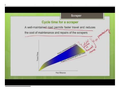
And for every individual section, you are supposed to determine the speed and the travel time. This picture clearly shows like what are the benefits we get by maintaining the haul route. This is just a schematic picture which shows how well maintained road permits faster travel and it reduces the cost of maintenance and the repair of the machine also. If you maintain your haul route, you can increase your life of a machine.
