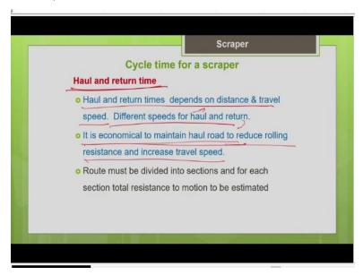
So, the next important component of the cycle time of the scraper is your haul and return time, as I told you it is a variable time, it is going to depend upon your travel distance and the speed of your machine. So, that speed depends upon your project site condition underfoot conditions. So, haul and return time depends upon the distance and the travel speed. So, we can see that obviously,
