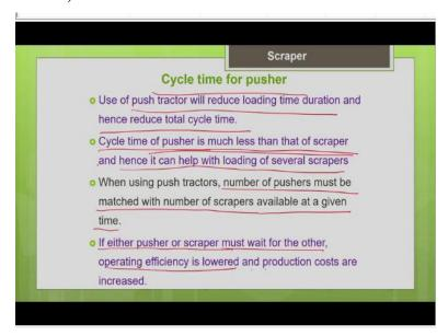
So, as we discussed earlier when you use a pusher for assisting your scraper, you can reduce the loading time of the scraper, it will help you to increase the productivity of the scraper and reducing unit production cost of the scraper. So, use a push tractor will reduce the loading time duration and hence reducing total cycle time and another important thing to be noted is the cycle time of the pusher is much less than that of the scraper.
