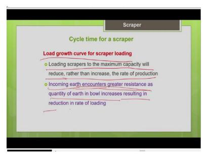
Another important concept which we need to know is about the load growth curve for scraper loading. So, we commonly believed that when we load this scraper when we fill the bowl of the scraper to the maximum capacity we are going to maximize a production. So, this is what is a common belief this is what is a common assumption, but that is not true. So, people have done the studies and they proved that when we tried to load the scraper to its fullest capacity.
