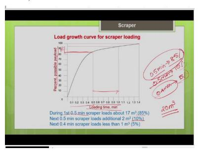
See, you have the loading time in minutes in the x axis and you have the percentage possible payload in the y axis. So, possible payload in percentage means what is the maximum capacity of your bowl? So, how much you actually fill your bowl? So, that percentage will be plotted here. So, now you can say that during the first 0.5 minute say the scraper capacity is 20 m<sup>3</sup>. The maximum capacity of the scraper which we have considered here is say 20 m<sup>3</sup>.
