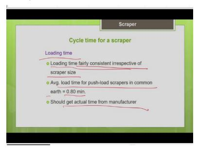
So, basically the loading time of the scraper is fairly consistent irrespective of the scraper size. So, that means whether it is going to be a smaller scraper or bigger scraper in both cases. So, commonly we can say that we are going to assist this scraper with the help of a pusher according to the size of the scraper the compatible size of the pusher you have to select and we are going to supplement the loading power.
